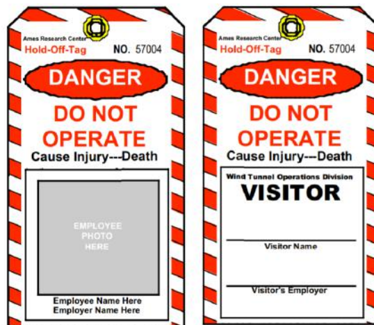
Figure 58. Employee and visitor lockout tagout measures, Personal Danger Tags (Do Not Operate) as shown in the AMES Safety Manual.
