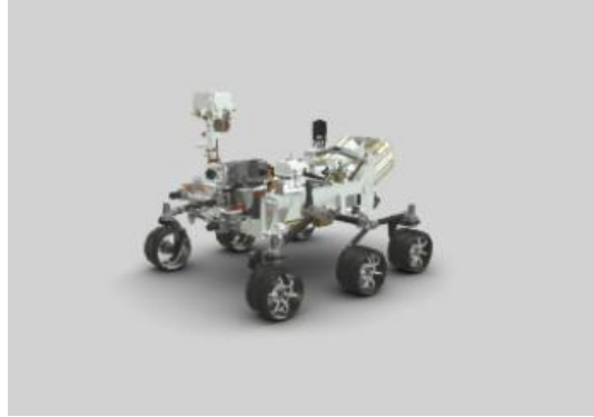
Figure 8. Digital model of Perseverance, a larger form rover which is powered via RTG and designed by the Jet Propulsion Laboratory.
