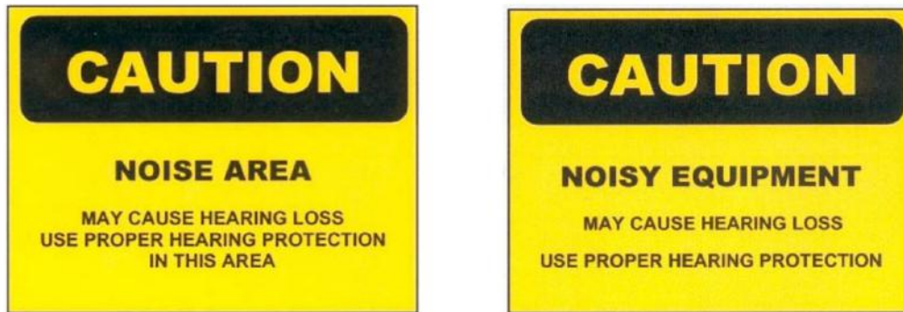
Figure 60. Black and yellow Noise caution signs are mandatory in work areas with the potential for causing hearing damage as shown in the AMES Safety Manual.
