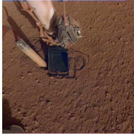
Figure 10. In this image from Oct. 26, 2019, the InSight Mars lander's heat probe, or "mole," is seen after backing about halfway out of the hole it had burrowed. (Image credit: NASA/JPL-Caltech). Science.com
