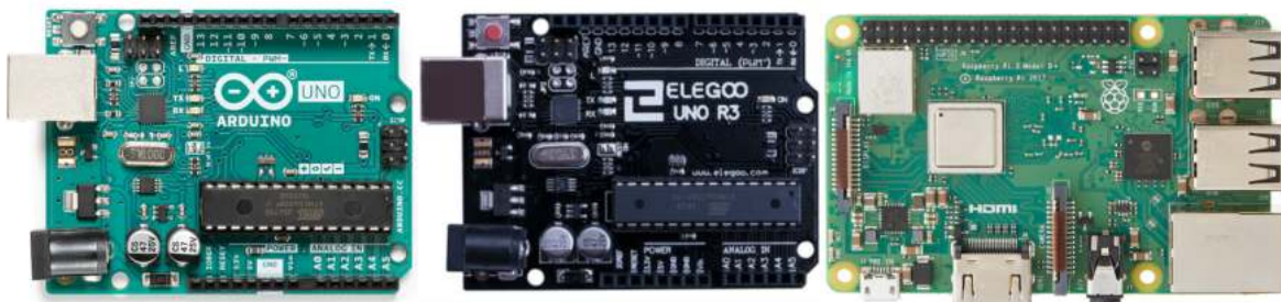
Figure 3.3.7-1: Microcontrollers Left to Right - Arduino Uno R3, Elegoo Uno R3, Raspberry Pi 3
