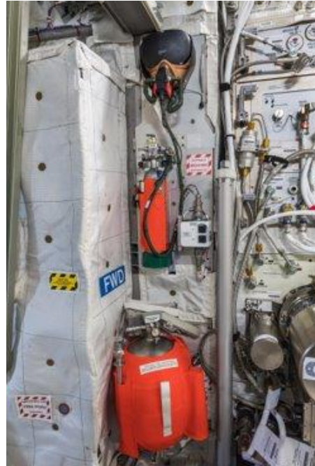
Figure 4.1.5-1 PBA and PFE aboard the Columbus that are equipped on the Mars EEV
